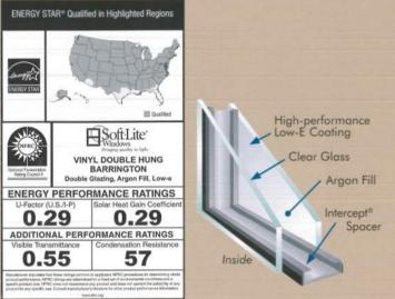
Above values are for a Barringtong double-hung window with Low-E Plus, featuring single-strength glass, Intercept spacer, argon gas, and without grids
