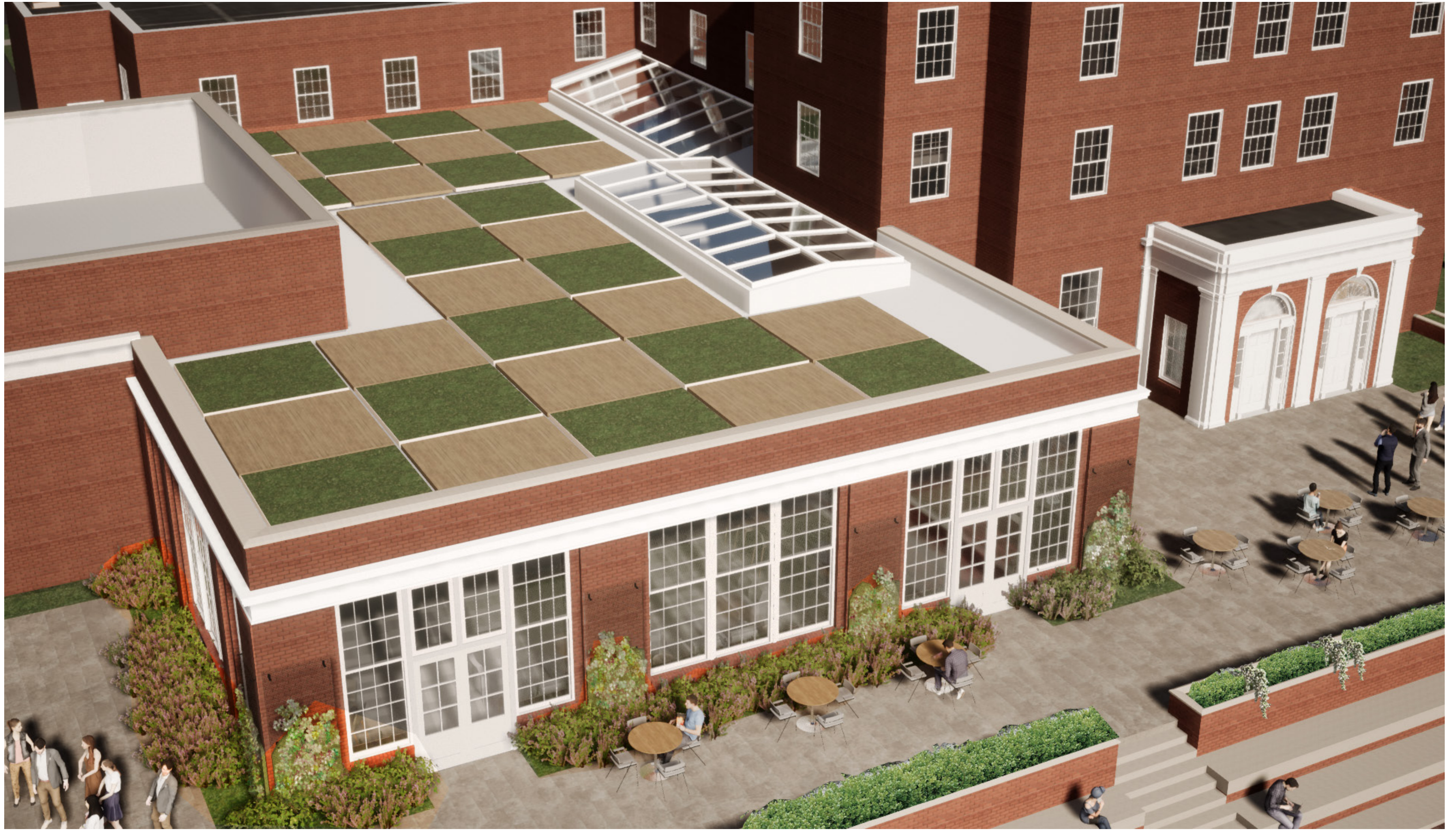
VIEW OF GREEN ROOF
