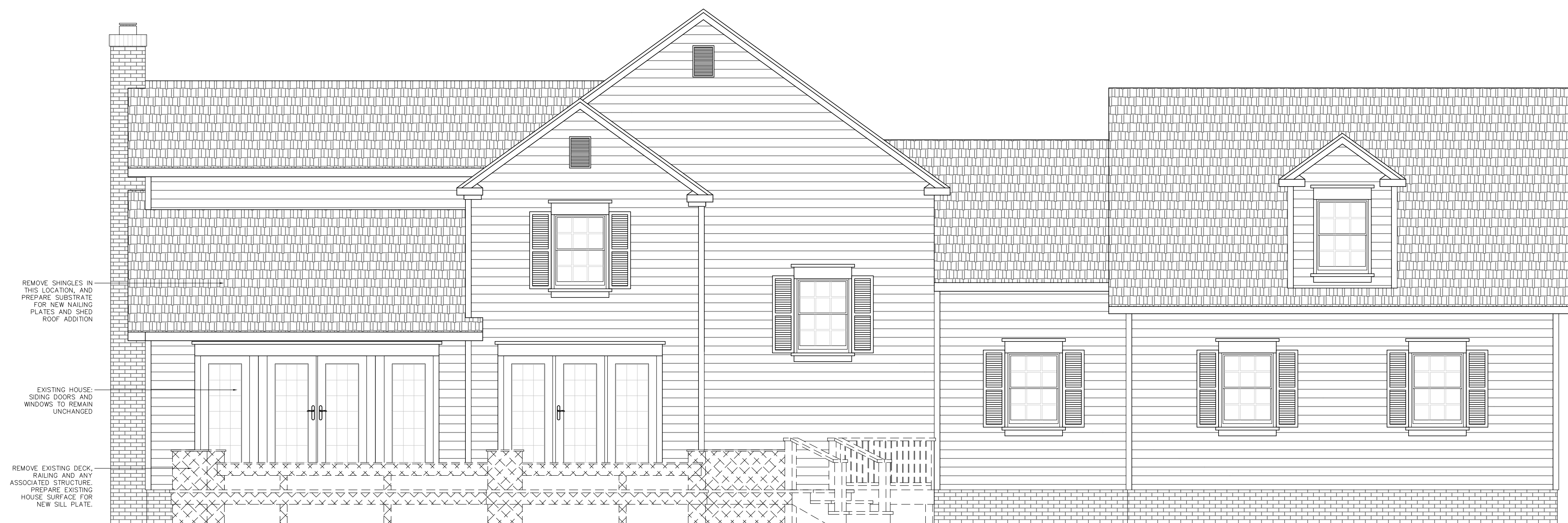
1 EXISTING REAR ELEVATION - DECK DEMOLITION SCALE 1/4" = 1'-0"
