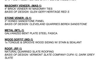
ALUMINUM STOREFRONT: (SF-1) ALUMINUM FRAMED ENTRANCES AND STOREFRONTS. BASIS OF DESIGN: KAWNEER TRIFAB 451 ALUMINUM WINDOWS: (SF-2) ALUMINUM DOORS AND FRAMES. BASIS OF DESIGN: GRAHAM GT6700 & GT7700 RUBBER ROOF: (RF-1) RUBBER ROOF MEMBRANE (TPO OR EPDM) O/ 19/32" APA RATED EXTERIOR GRADE SHEATHING/ MINIMUM SLOPE 1/4" PER FOOT. COORDINATE SELECTION WITH ARCHITECT AND OWNER
