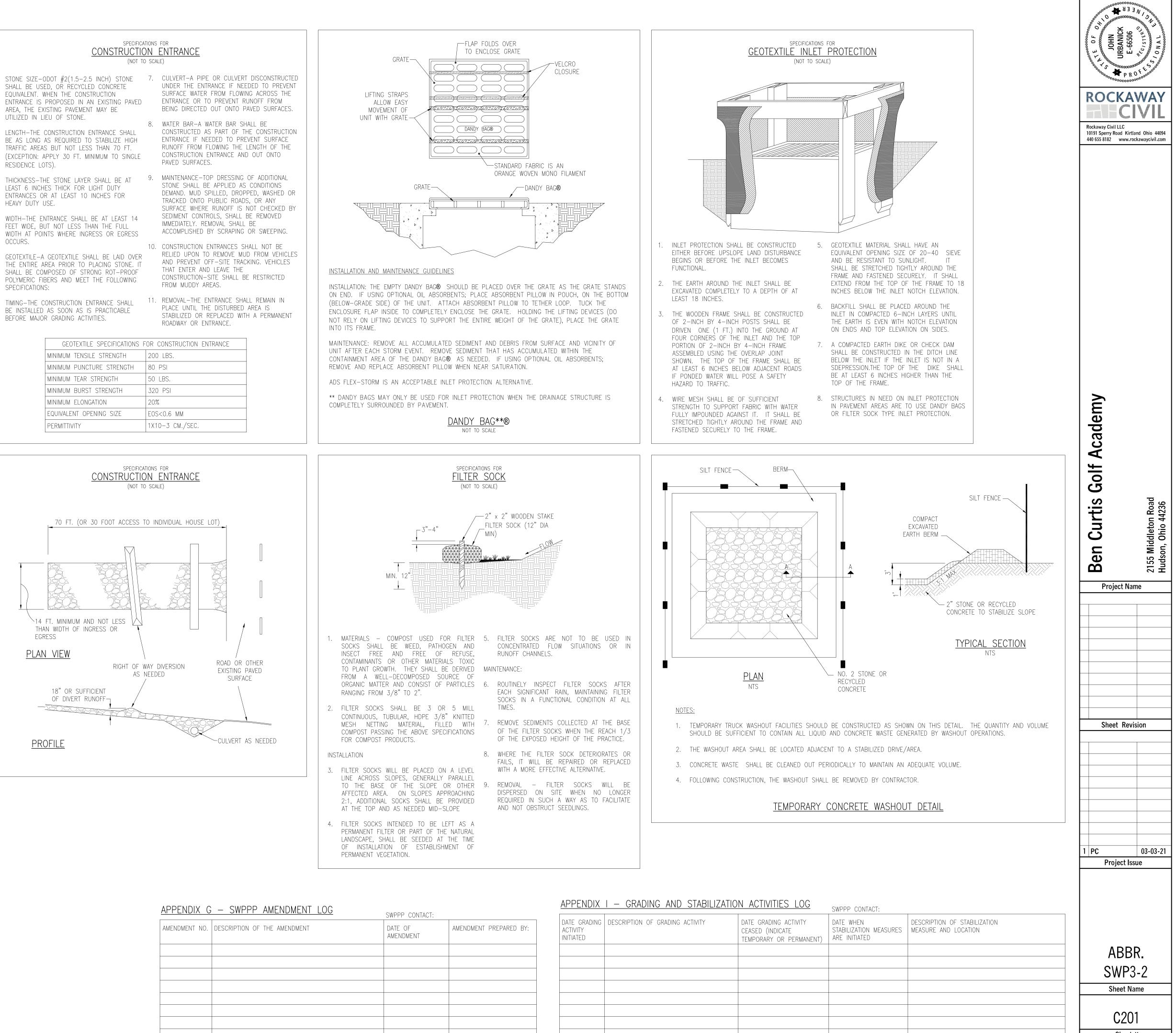
SHALL BE USED, OR RECYCLED CONCRETE EQUIVALENT. WHEN THE CONSTRUCTION AREA, THE EXISTING PAVEMENT MAY BE UTILIZED IN LIEU OF STONE.
