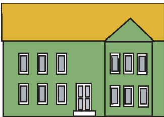
(42) Seven Asymmetrically Bays with Centered Front Door
