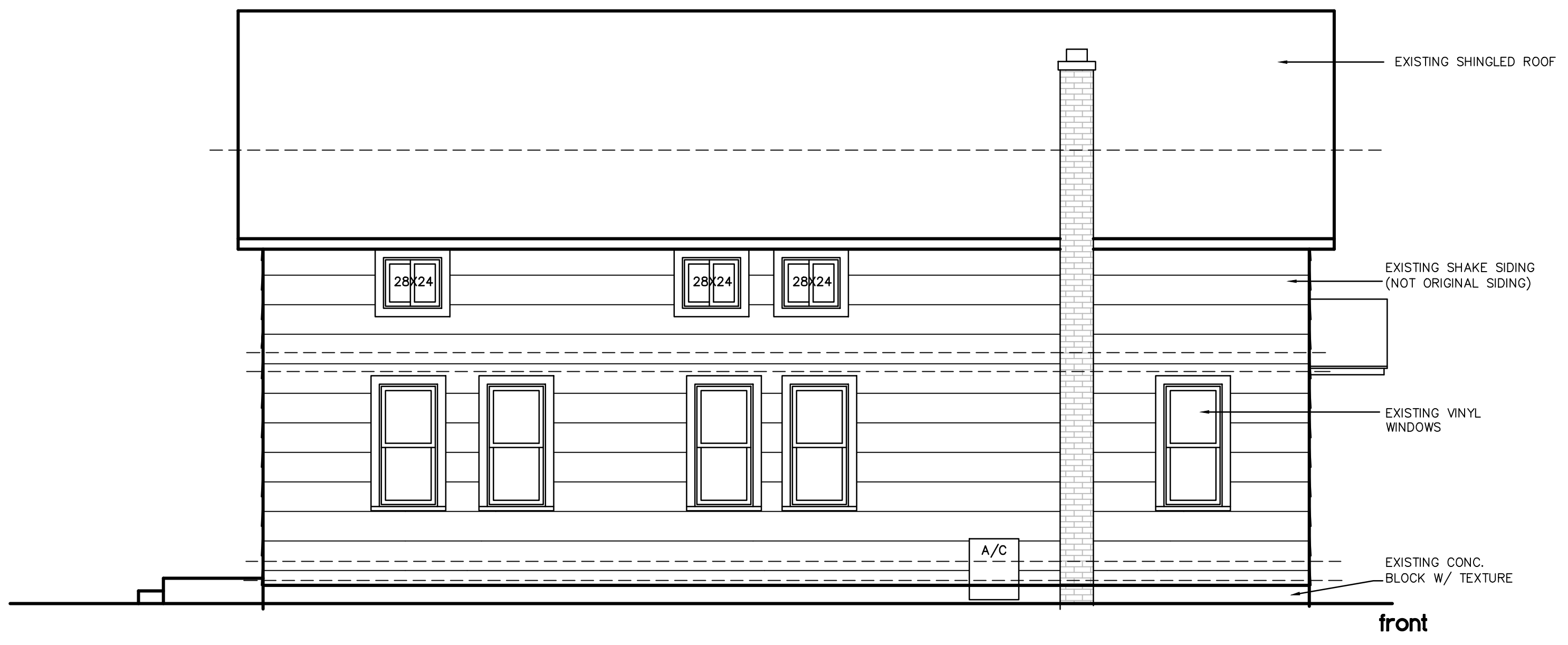
EXISTING LEFT ELEVATION WEST SCALE : 1/8" = 1'-0"
