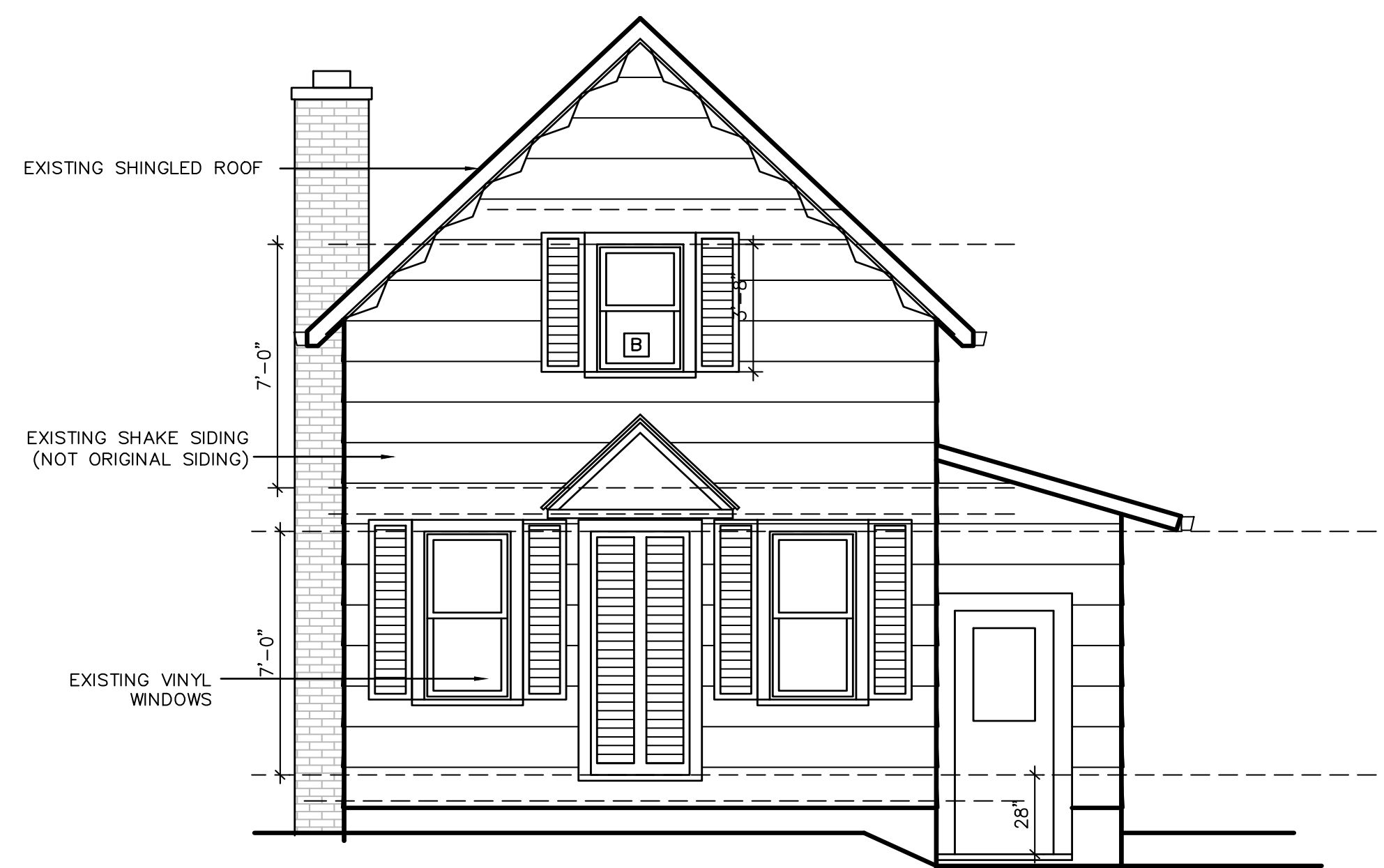
EXISTING FRONT ELEVATION NORTH SCALE : 1/8" = 1'-0"
