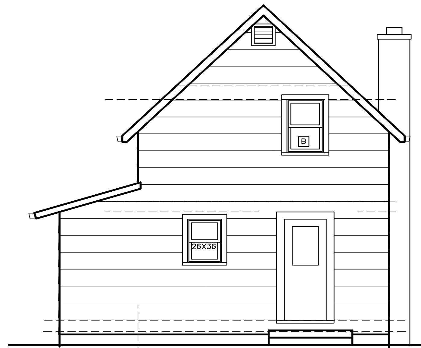
EXISTING REAR ELEVATION SOUTH SCALE : 1/8" = 1'-0"
