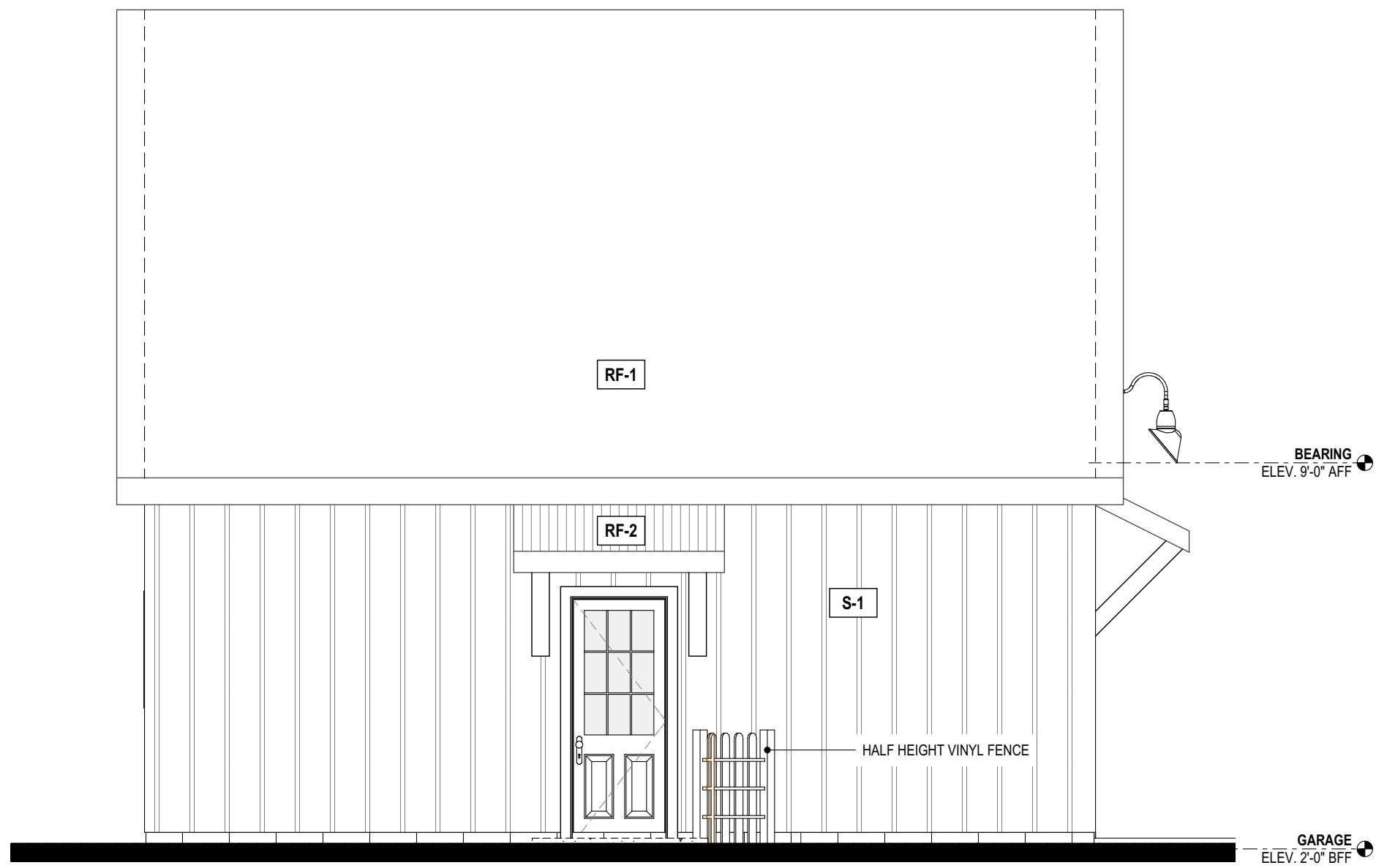
2 SIDE OF ACCESSORY BUILDING ELEVATION (WEST) SCALE: 1/4" = 1'-0"
