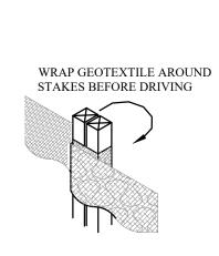
JOINING SECTIONS OF SILT FENCE DETAIL
