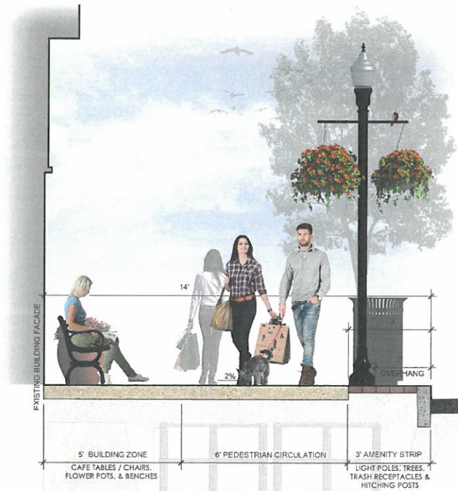
TYPICAL SIDEWALK SECTION
