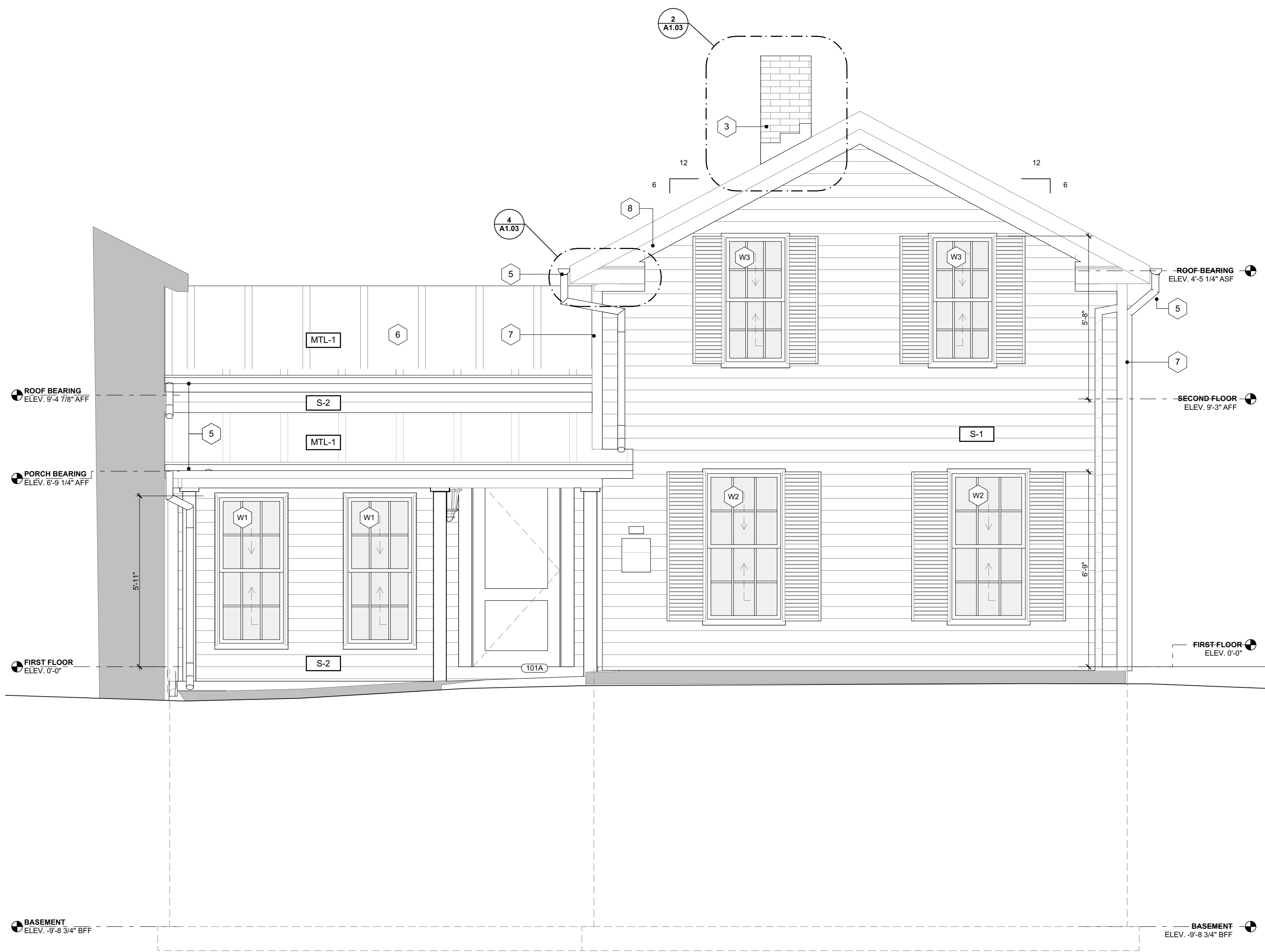
1 EXTERIOR ELEVATION - WEST (FRONT OF THE BUILDING) SCALE: 3/8" = 1'-0"
