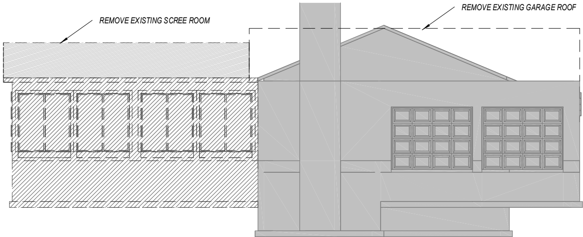
11 DEMO -LEFT ELEVATION 3/32" = 1'-0"
