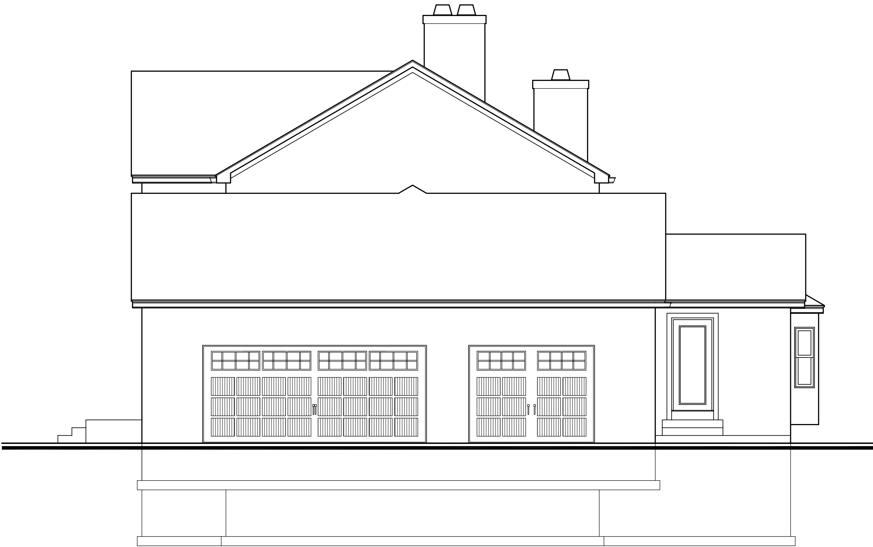
RIGHT SIDE ELEVATION - EXISTING S: 1/4" = 1'-0"
