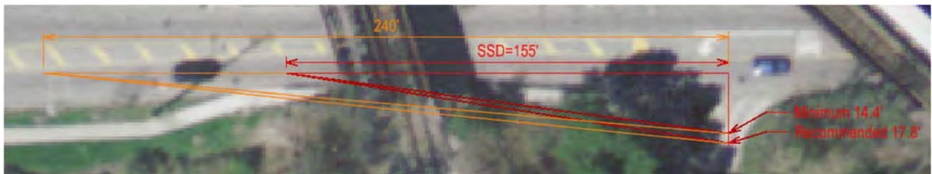
Figure 3: Sight distance details
