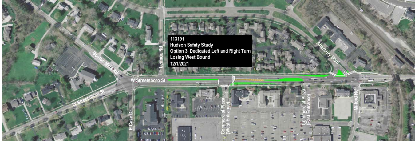
Figure 6: Segment – Boston Mills Rd / E Case Dr To to Atterbury Blvd Recommended Lane Configuration (Option 3)
