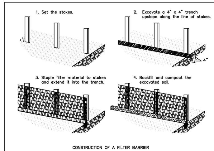
Source: Installation of Straw and Fabric Filter Barriers for Sediment Control, Sherwood and Wyant
