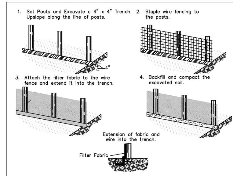
Source: Adapted from Installation of Straw and Fabric Filter Barriers for Sediment Control, Sherwood and Wyant
