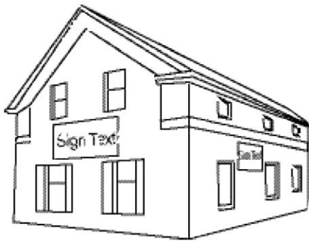
47 Awkward placement of sign panels.
