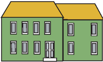
(41) Four Symmetrical Bays with an Asymmetrical Front Door
