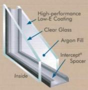
Above values are for a Barringtong double-hung window with Low-E Plus, featuring single-strength glass, Intercept spacer, argon gas, and without grids.
