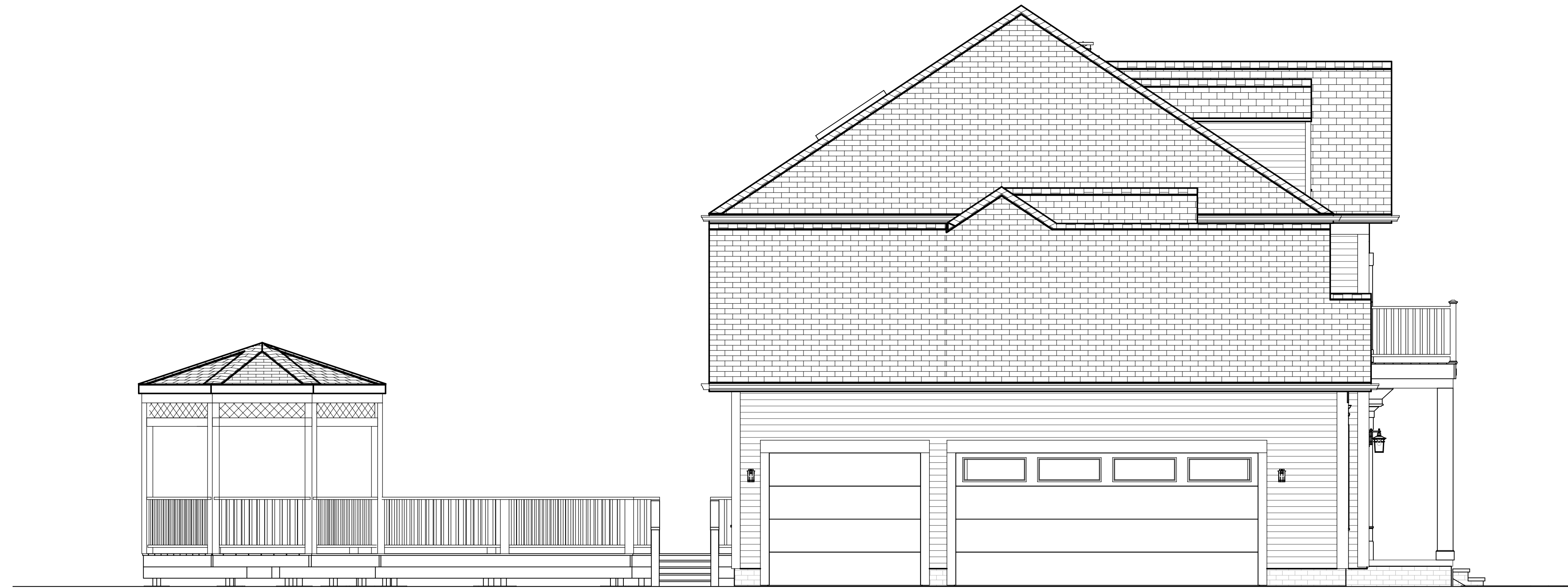
② LEFT SIDE EXISTING/DEMO ELEVATION 1/4" = 1'-0"
