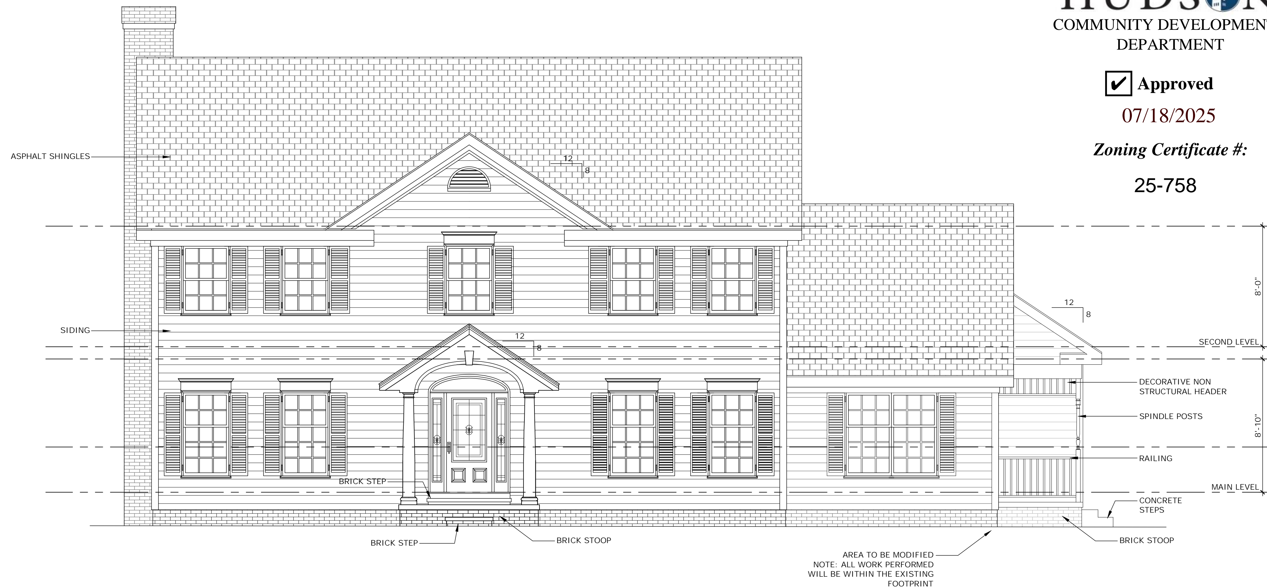
1 EXISTING FRONT ELEVATION SCALE: 1/4" = 1'-0"
