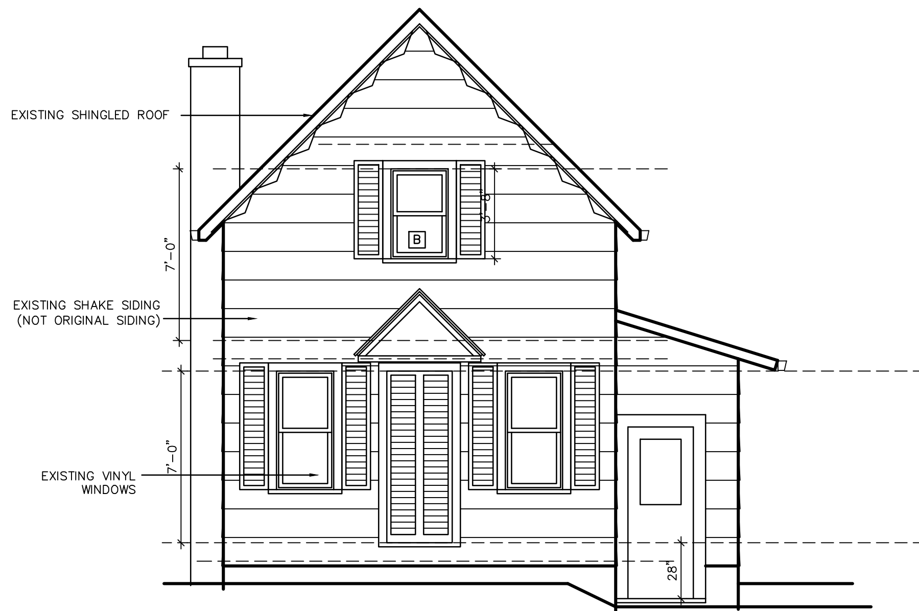
EXISTING FRONT ELEVATION
