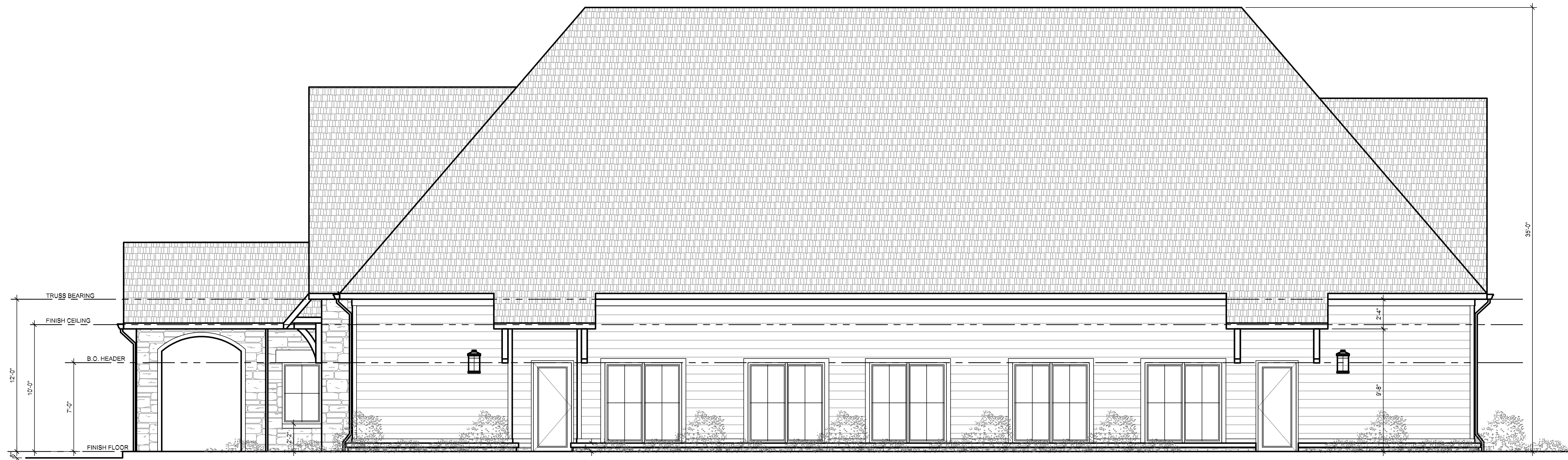
3 PROPOSED REAR ELEVATION SCALE: 1/4" = 1'-0"
