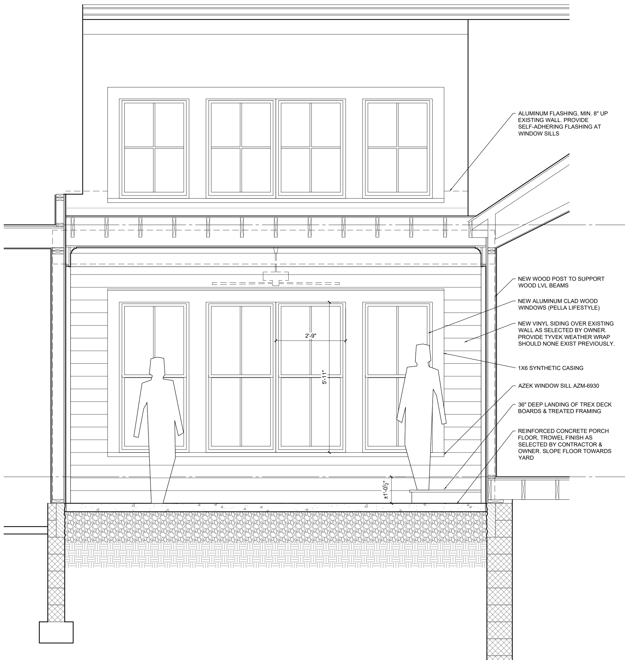
2 BUILDING SECTION SCALE: 1/2" = 1'-0"
