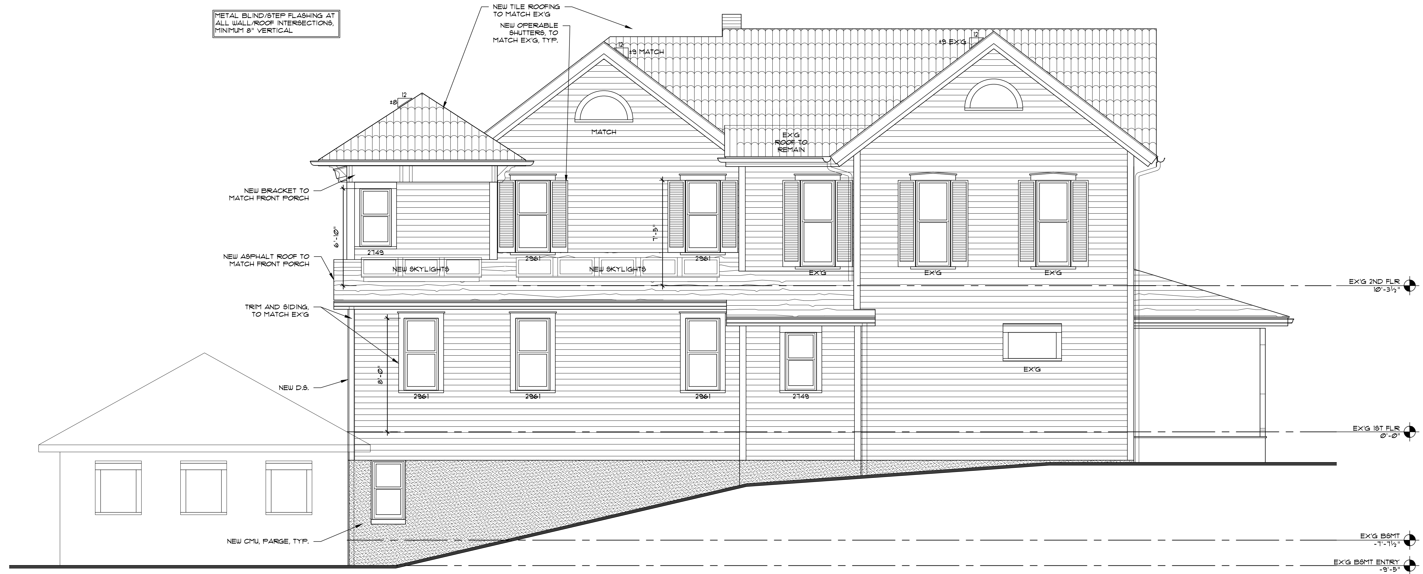
2 Proposed Side Elevation (NE) 1/4" = 1'-0"
