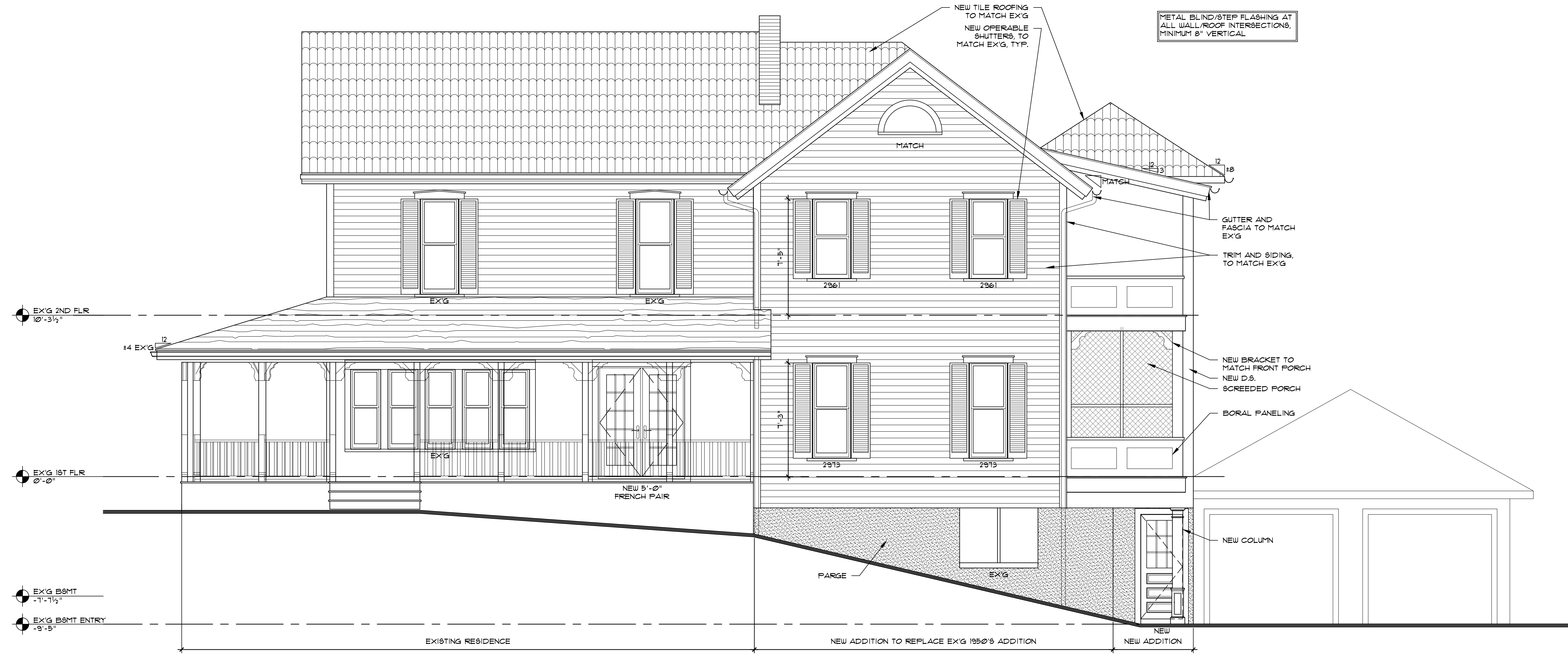
2 A-6 Proposed Side Elevation (SW) 1/4" = 1'-0"
