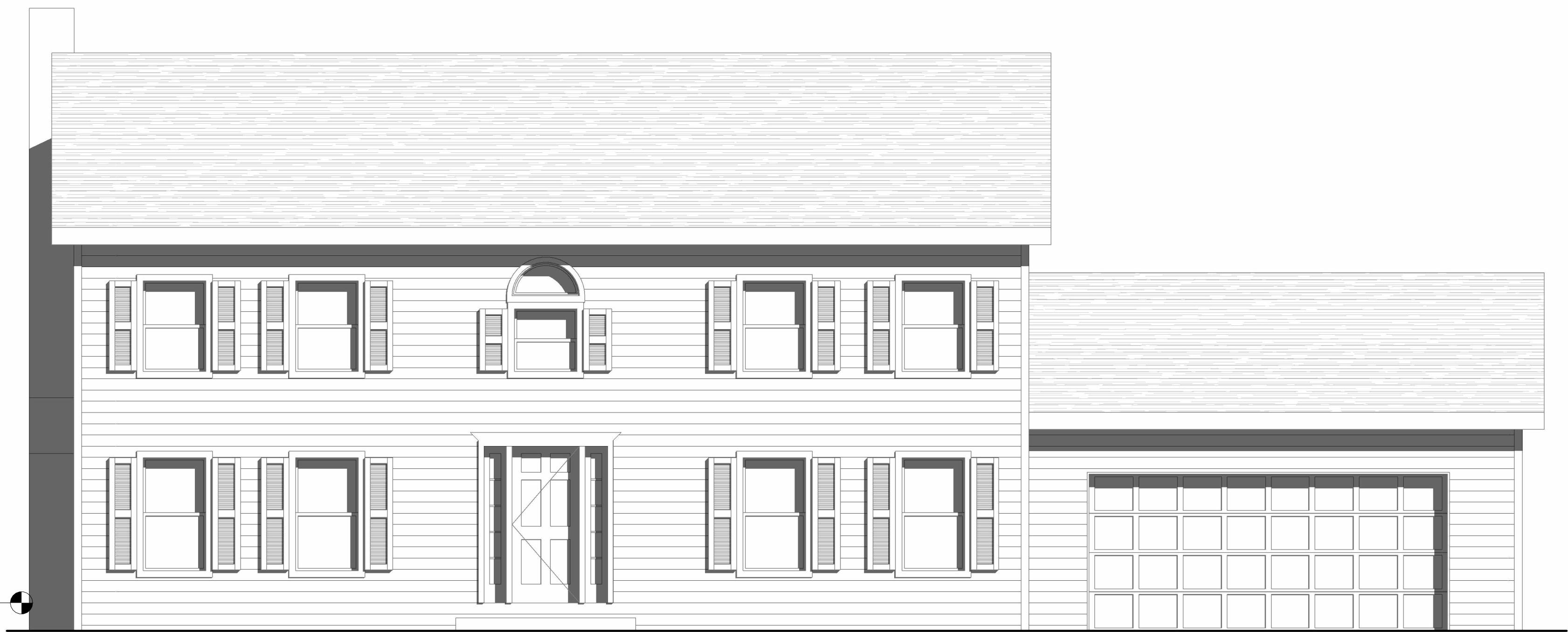
② FRONT ELEVATION - NORTH 1/4" = 1'-0"
