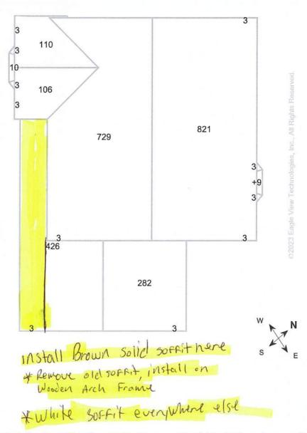
Note: This diagram shows the square feet of each roof facet (rounded to the nearest Foot). The total area in square feet, at the top of this page, is based on the non-rounded values of each roof facet (rounded to the nearest square foot after being totaled).
