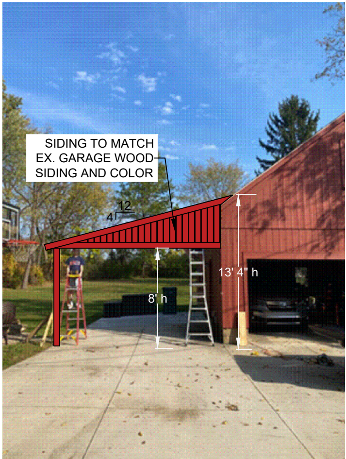
3 4 PROPOSED WEST GARAGE ELEVATION SCALE: 1/8"=1'
