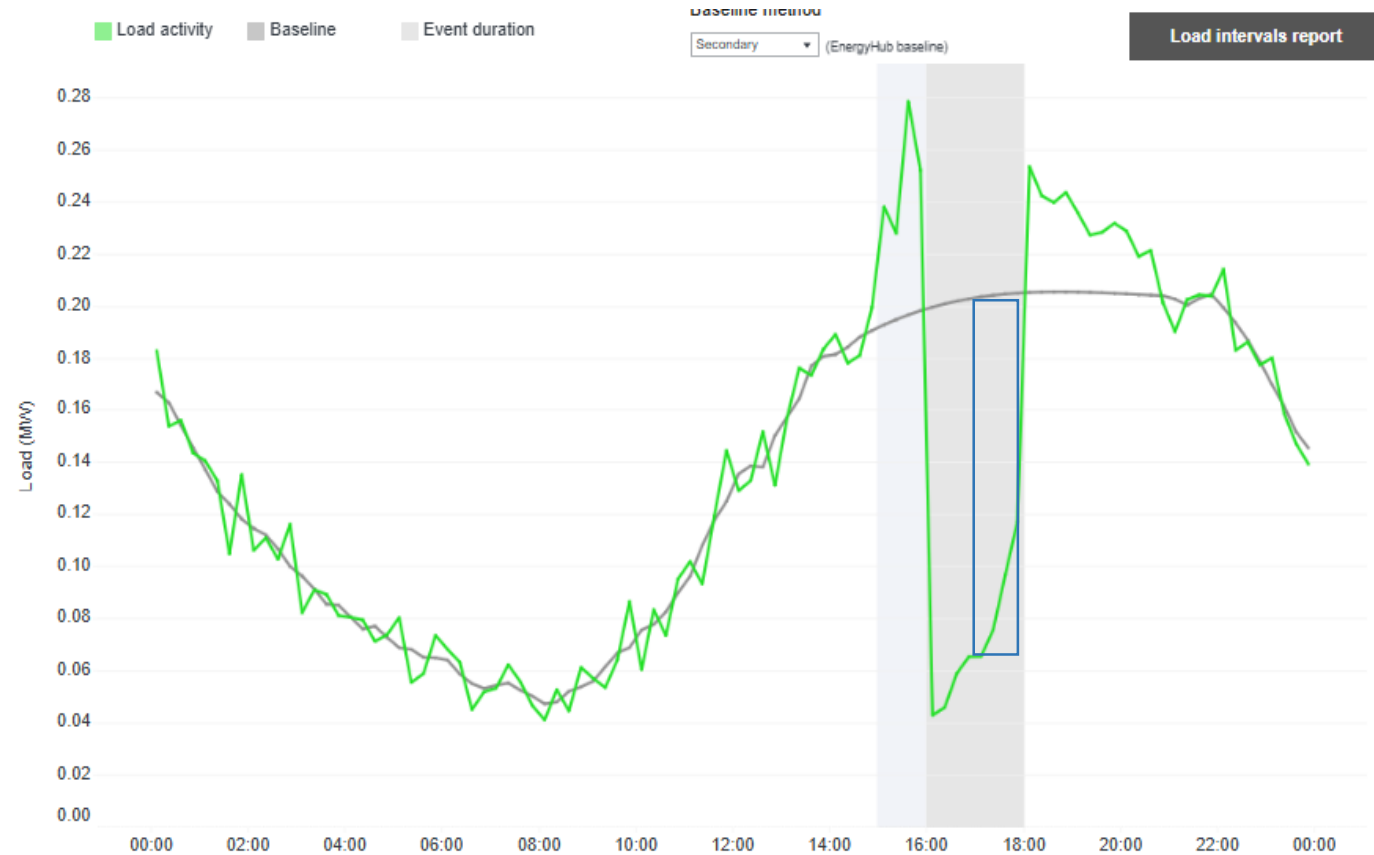
Sample Event: baseline is the gray line; event duration gray block shows one-hour precool, two-hour event; green line illustrates the AC load. The load shed was 1.23 kilowatts (KW)/thermostat during the CP hour (the blue box HE 18), achieved 115.4 kW total load shed for CP hour. The load spike before the event is due to precooling; the load spike after the event is from the AC load coming back online.
