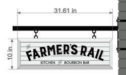
Cedar wood plank construction with face frame and full return to cover edges of sign. Distressed painted finish and hand painted graphics in matte finish
