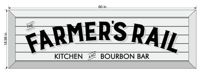
Cedar wood plank construction with face frame and full return to cover edges of sign. Distressed painted finish and hand painted graphics in matte finish.
