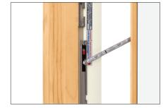
Limits the casement sash opening to less than 4 inches when engaged. The release mechanism allows for operation beyond 4 inches. This option meets the ASTM F2090-21 standard.
