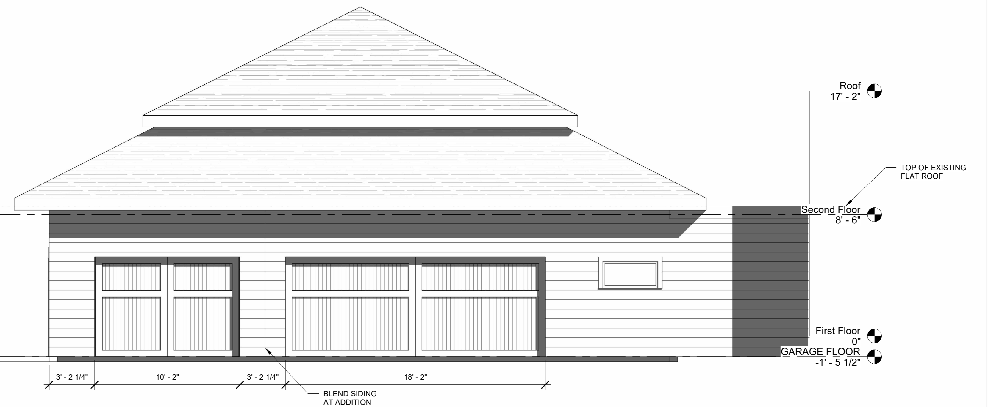
② SIDE ELEVATION - GARAGE DOORS 1/4" = 1'-0"
