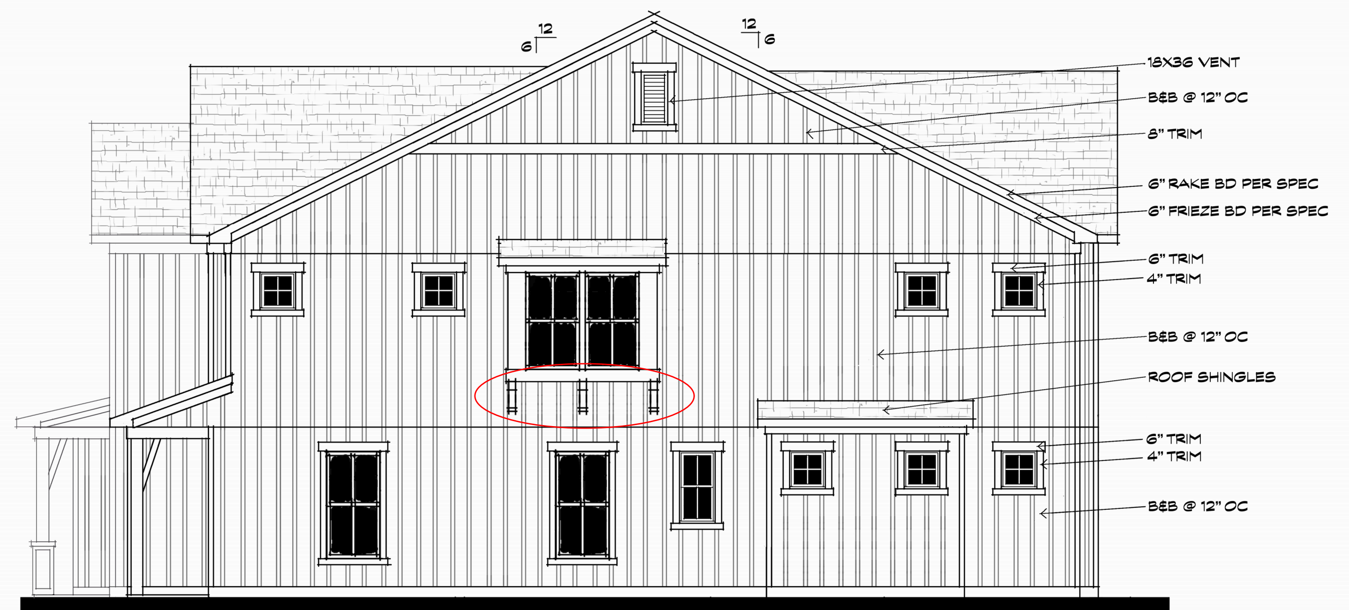
RIGHT SIDE ELEVATION - FARMHOUSE SCALE: 3/16"=1'-0"
