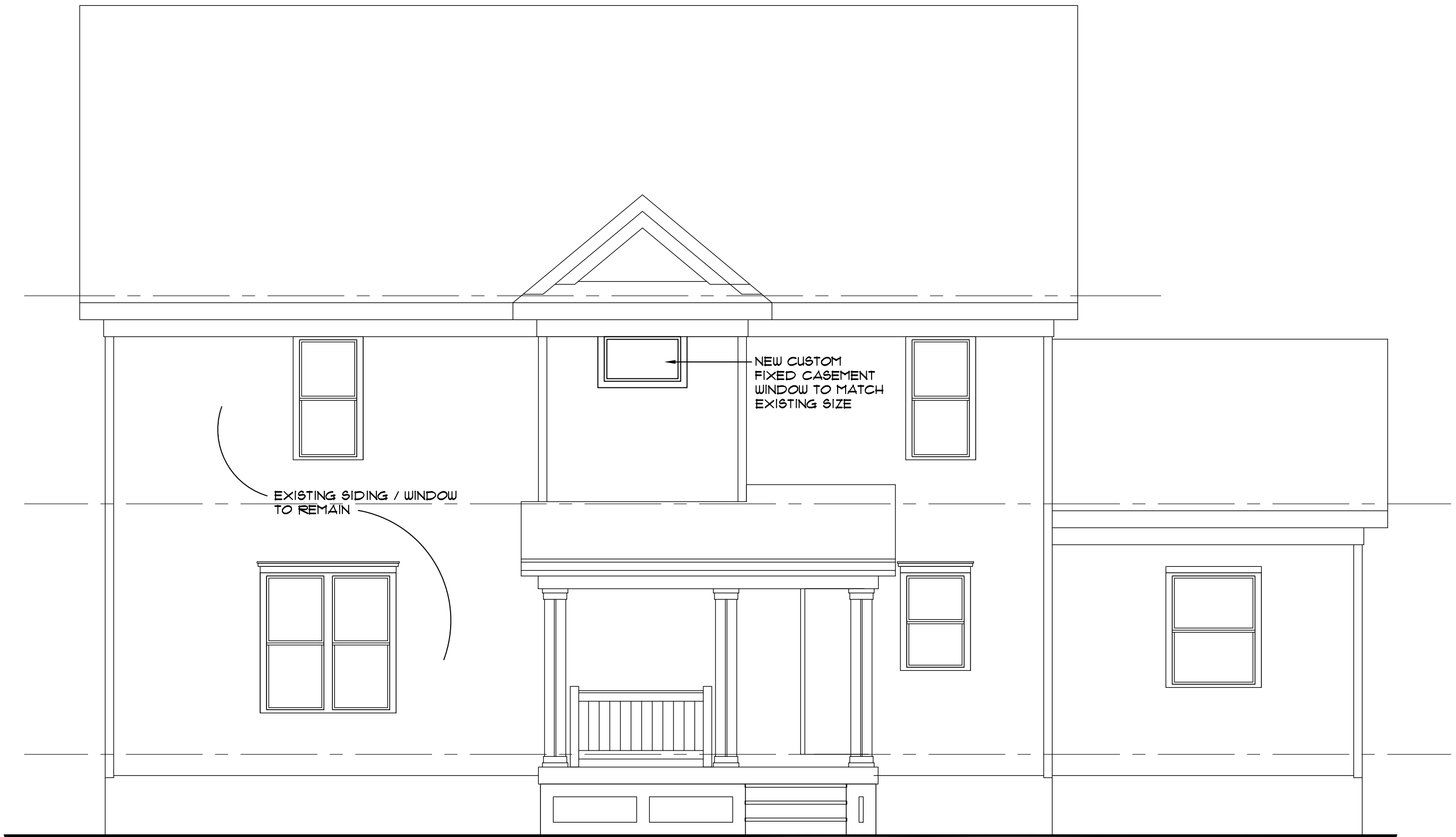
EAST ELEVATION SCALE: 1/4" = 1'-0"
