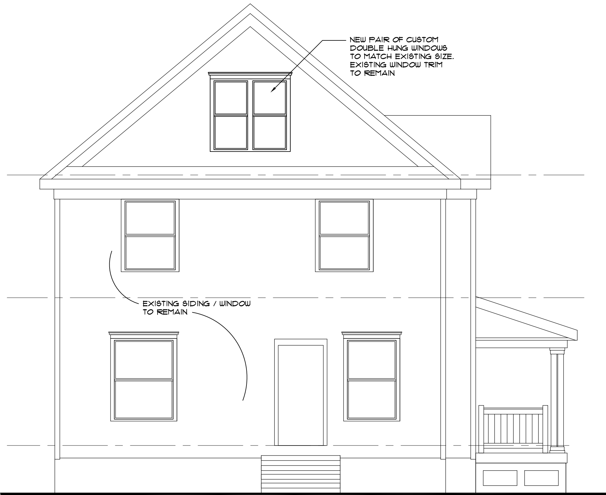
SOUTH ELEVATION SCALE: 1/4" = 1'-0"
