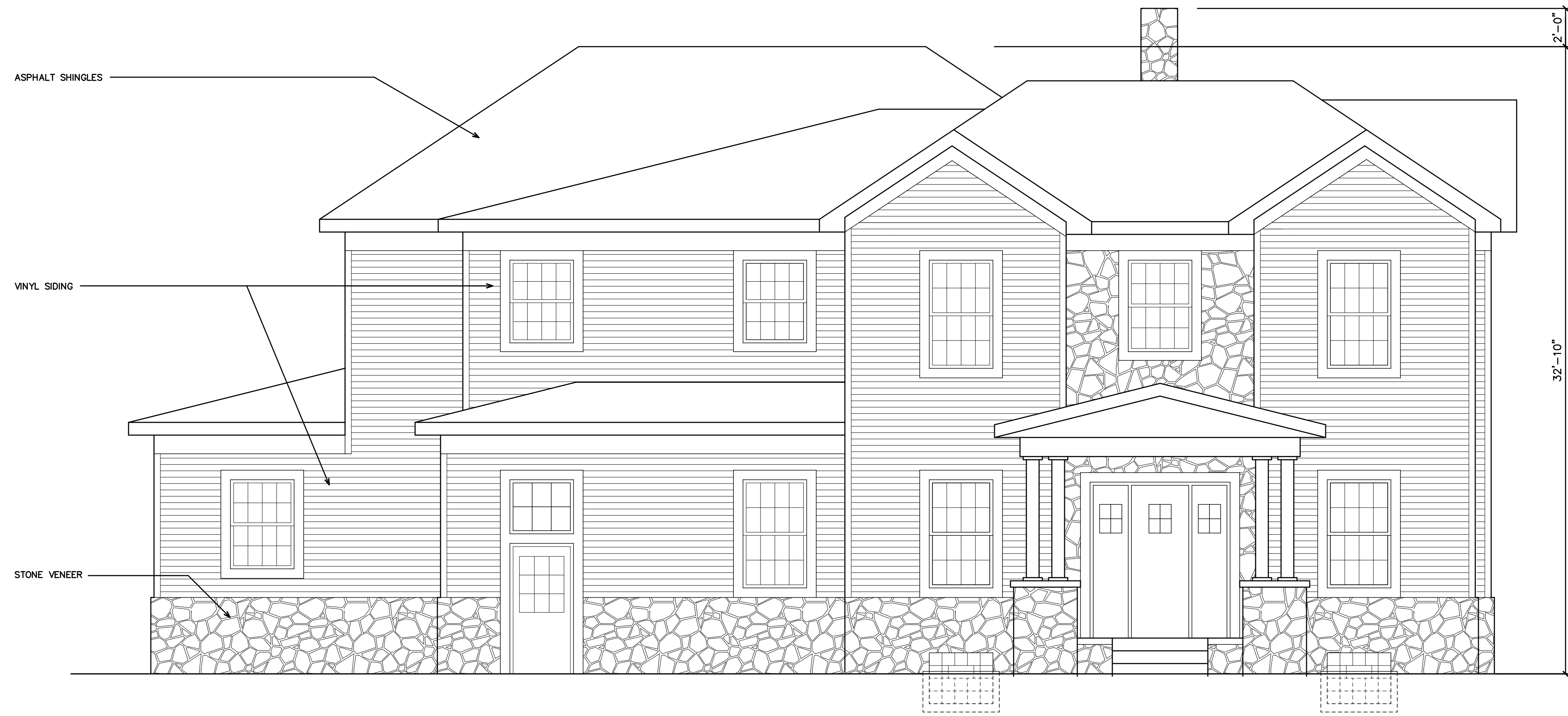
NORTH ELEVATION SCALE 1/4" = 1' - 0"
